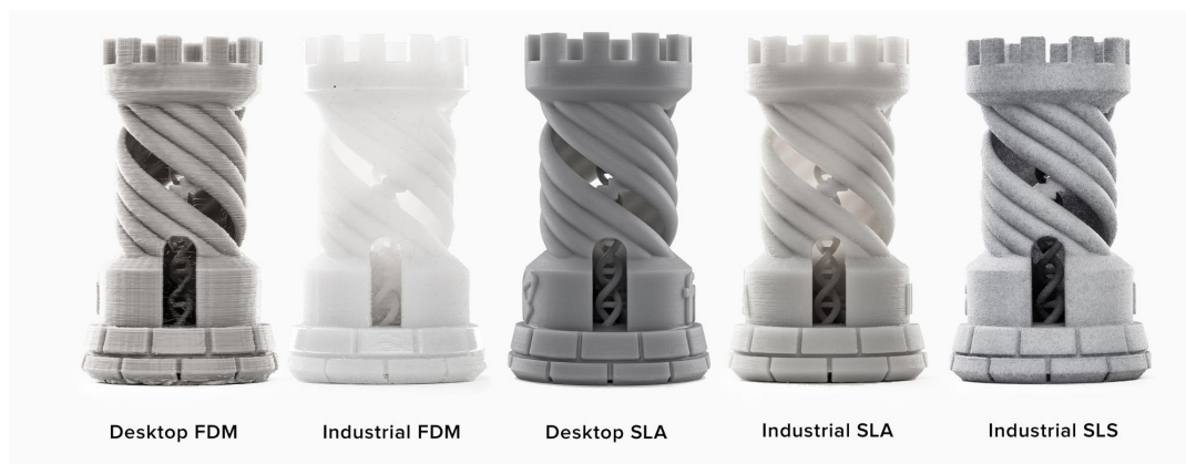
Rooks printed at 100 micron layer height on an desktop and industrial FDM, desktop SLA (Form 2), industrial SLA and industrial SLS 3D printers.
