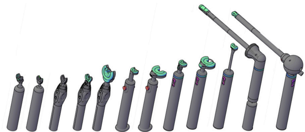
Consecutive iterations of Sutru , an automated surgical suturing device prototyped on Formlabs SLA printers.
